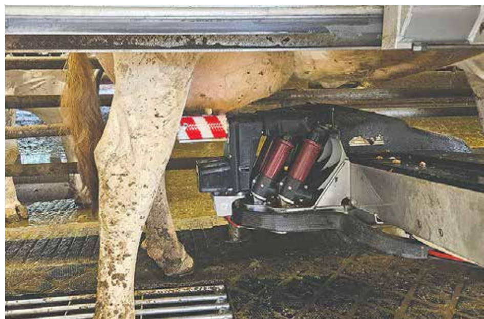
Brushes clean and laser-guided tubes do the milking.
